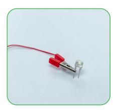
Attach the LED horizontally on the battery holder. Make the battery holder stand upright and use it as a stand
