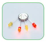
THE TWO LEGS OF AN LED ARE UNEQUAL. WHY DO YOU THINK IT IS SO? DOES IT MAKE A DIFFERENCE WHEN CONNECTING AN LED TO A COIN CELL?
